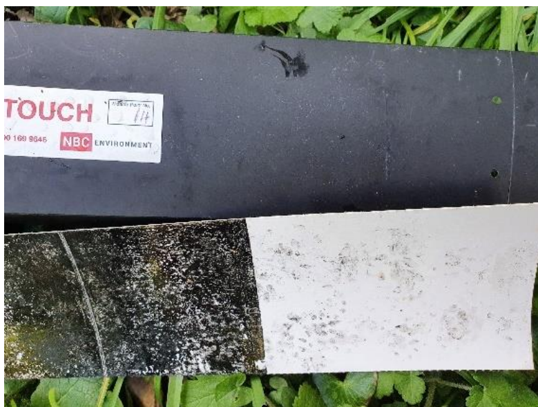
Figure 8. Photograph showing rodent footprints on ink plate.
